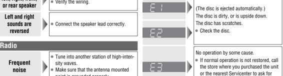
Make sure that the antenna mounted noise point is grounded properly.
